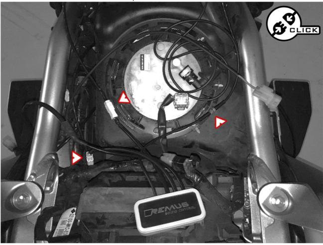
Guide the single-pole plug to the right and the three-pole plug to the left side of the vehicle, to the respective plug connections. You will find these behind the previously removed side panels.
