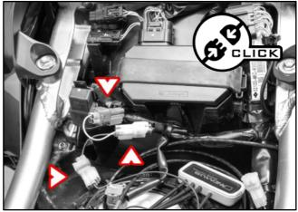
Connect the cables of the actuators and flap control button to the REMUS control unit.
