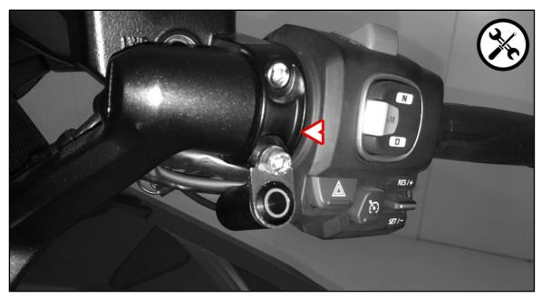
Guide the control cable along the motorcycle, as shown on the picture.
