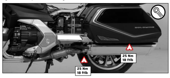
Remount all previously removed parts and fix all cables by using cable ties.
