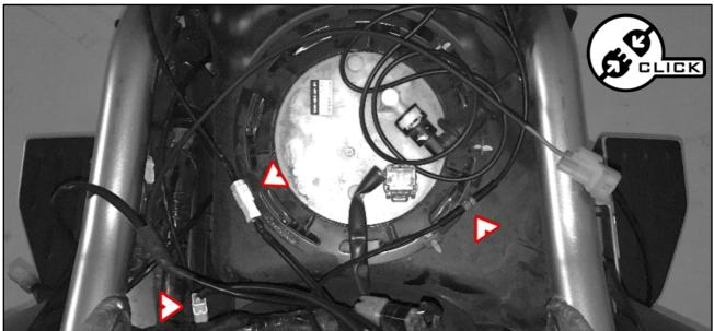
Guide the three-pole plug to the left side of the vehicle, to the respective plug connection. You will find these behind the previously removed side panels.
