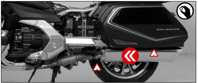
Guide the actuator cables of the actuators as shown in the picture.
