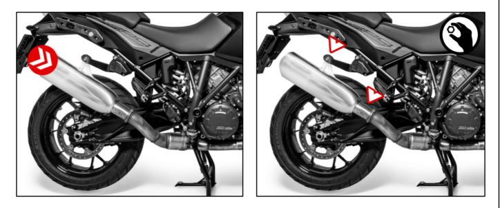
Align the REMUS sport exhaust and tighten the connections. Mount the REMUS heat shield onto the muffler.
