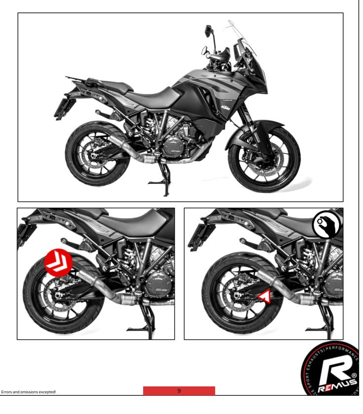
Mount the supplied bracket on the REMUS sport exhaust. Slip the sport exhaust onto the connection tube, screw the bracket and hook the spring.
