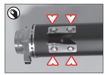
Remove the stock bracket and mount it onto the REMUS sport exhaust.
