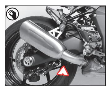
Align the REMUS sport exhaust and tighten the connections.
