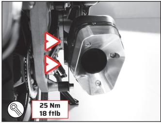
Hang in the spring. Align the REMUS sport exhaust and tighten the connections.
